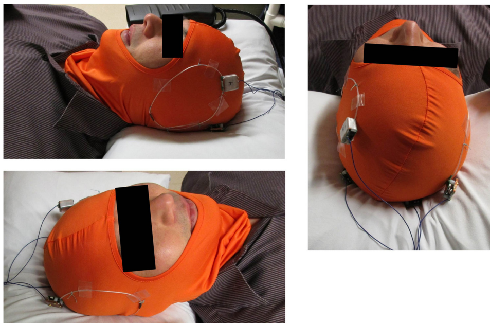
Figure 3. Balaclava with four AIR coil elements placed on a normal volunteer.
