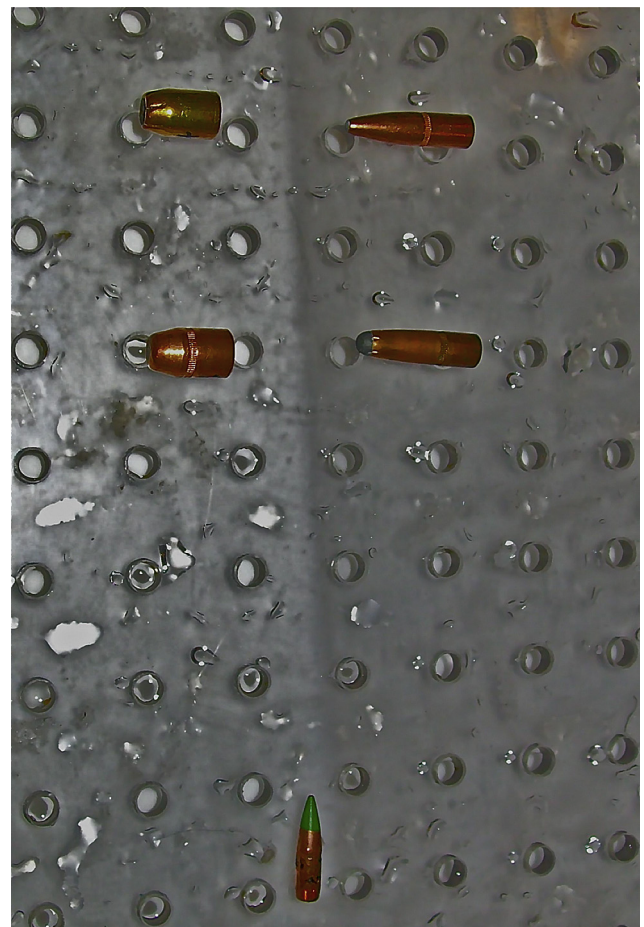
Fig. 5. Experimental setup for the evaluation of magnetic resonance imaging–related artifacts at 3-T. Note the five different bullets (Fig. 3) placed on the plastic frame, as follows: top row (left to right): Bullets 23 and 8; middle row (left to right): Bullets 25 and 10; and bottom row: Bullet 32.
