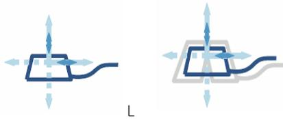
Left illustration shows a linear coil only sensitive to the vertical component of the field. The illustration on the right shows an addition of a butterfly element, providing sensitivity only to the horizontal component
