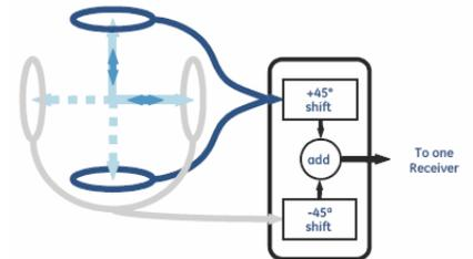
A quadrature combiner allows two quadrature channel signals to be received by one receiver.
