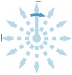
The net field vector can be resolved into two orthogonal (right angle) oscillating vectors. These can be oriented in any direction in a plane orthogonal to the magnet's Z-axis as long as the two vectors remain orthogonal. When one vector is maximum, the other is minimum.
