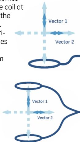
Two opposed linear coils can be connected together for more uniform coverage of the volume, but they are still only sensitive to one oscillating vector.
