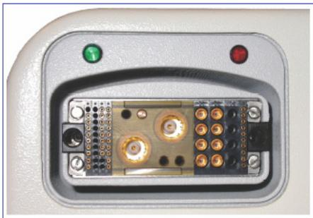
Coil indicator lights next to each coil port let you know when your coil connection is secure. When a coil
