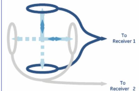
With Phased Array Coils, each quadrature channel is connected to a separate receiver channel.
