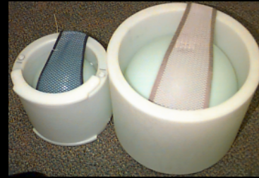
Head (16.8cm) and Body (26.6cm) Spheres with Loading Cylinders
