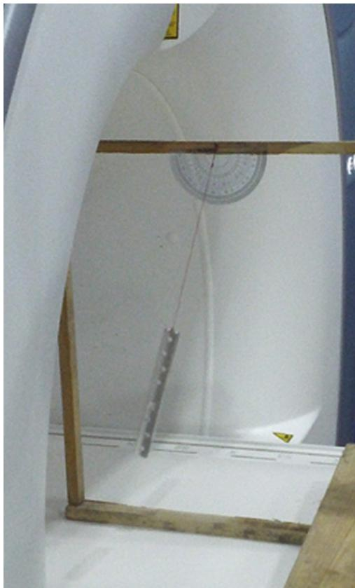
**Fig. 1.** Demonstration of the experimental setup used to assess hanging angle displacement of implants during an imaging sequence. (From Zou YF, Chu B, Wang CB, et al. Evaluation of MR issues for the latest standard brands of orthopedic metal implants: plates and screws. *Eur J Radiol* 2015;84(3):451; with permission.)
