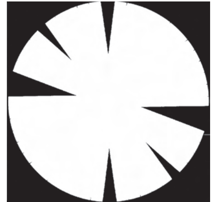
Figure 23. Several blades are completely thrown out during the final gridding process, which fills in only the white region of k-space. Data were collected from a healthy volunteer who rotated her head \pm 90^\circ during data acquisition.
